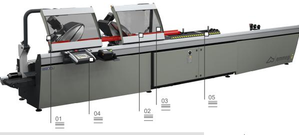
Twin-head cutting-off machine with 3 axes controlled by automatic movement of the mobile head and electronic management of all 45° (internal) to 15° (external) angles, with a precision, within each degree, of 280 positions.
